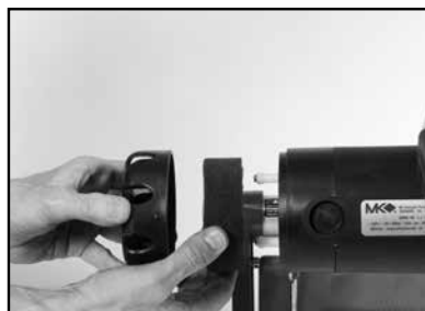
(B) Remove Motor Filter Cap from Filter Cap.
