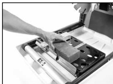
(B) Position masonry piece. Set against Cutting Guide and Ruler/Stop.
