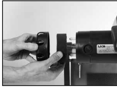
(B) Inspect Motor Air Filter for cleanliness.
