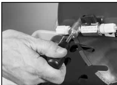
(B) Remove screw fitting.
