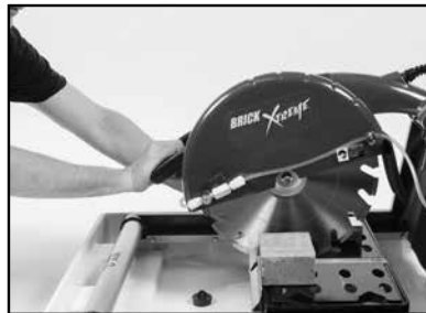
(B) Lower Cutting Head to begin cutting.
