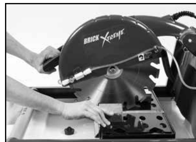
(C) Slowly push piece toward blade to cut. Turn OFF saw.
