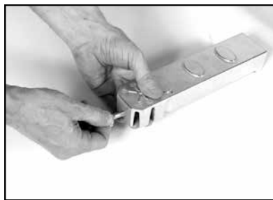
(A) Loosen Thumbscrew. Position adjustable Cutting Guide on Ruler/Stop.
