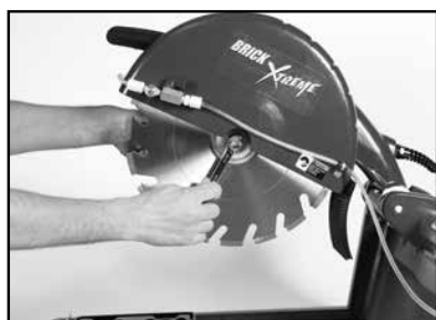
(A) Remove retaining screw and Outer Flange.
