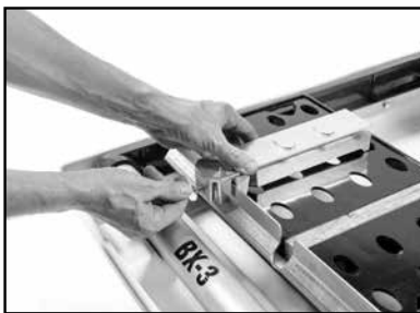
(B) Seat and tighten adjustable Cutting Guide.
