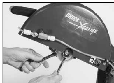
(A) Place wrenches on retaining screw and Inner Flange.
