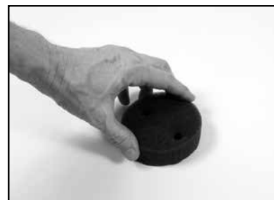
(C) Clean Filter by tapping on hard surface or using compressed air.
