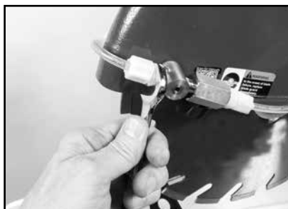
(A) Loosen tube fitting.
