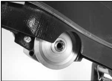
(A) Clean and lubricate Inner Flange and Motor Shaft.
