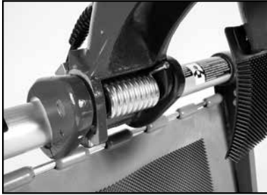
(A) Lubricate Cutting Head torsion spring.
