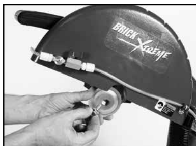
(B) Remove retaining screw and Outer Flange.
