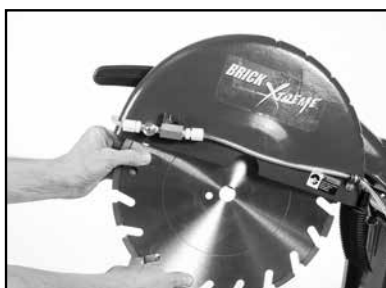
(B) Remove blade from Motor Shaft.
