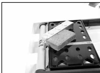
(B) Set material against adjust- able Cutting Guide and Ruler/Stop.
