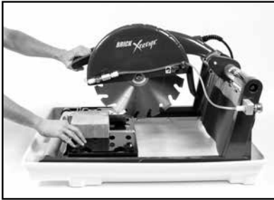
(A) Depress Trigger Switch to start cut.
