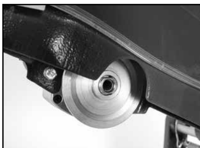
(B) Check for Roller Wheel damage.
