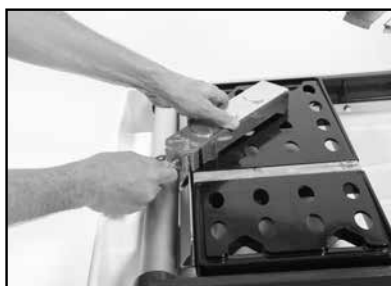
(A) Reposition adjustable Cut- ting Guide. Align 45° slots to Ruler/Stop.
