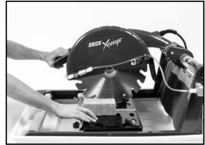
(C) Lower Cutting Head addi- tional 1/4 - 1/2 inch during pull stroke.
