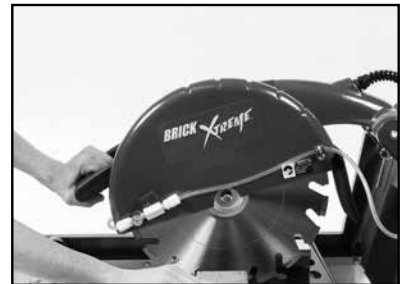
(C) Continue lowering head until cut complete. Turn OFF saw.
