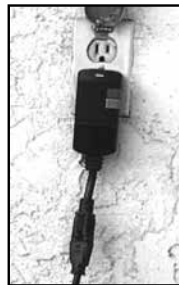
(B) Plug GFCI into Power Source.
