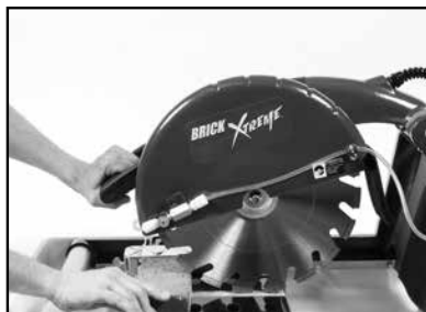
(B) Position work below Cutting Head.
