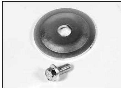
(B) Clean and lubricate blade retaining screw.
